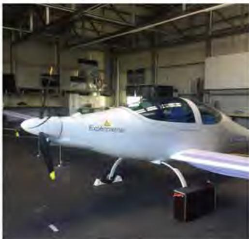
The single-engine SolarStratos plane has a weight of 450 kilograms, a length of 8.5 metres and a wingspan of 24.8 metres. The wings and other parts of the aircraft are covered with photocells, which occupy an area of 22 square metres. The plane is to rise to a height of more than 24,000 metres.
