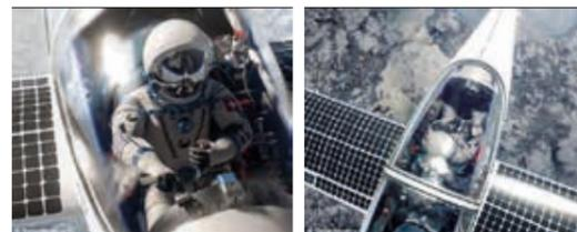
The plane is just 8.5 meters long and runs on a 32-kW electric engine and 20 kWh lithium-ion battery, charged by the craft's 22 square meter solar cells, which cover each wing
